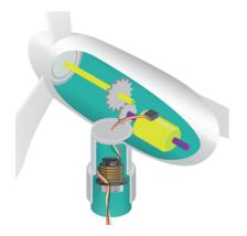
In this particular case, the energy generated by the small size and low voltage wind turbines from the electric generator (aboard the rotating pod) need to be transferred to the land. Slip ring are the best solution in order to avoid any cable twist while passing through the pylon.
